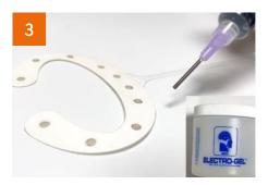
Using the syringe, draw up approximately 0.5cc of electrode gel and place the gel evenly on all electrodes (TMSi recommends the pictured Electro-Gel due to low impedances).
