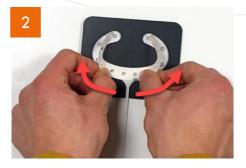
Take the double-sided adhesive, remove one of the white protective layers, and place the sticky side of the adhesive on the cEEGrid.
