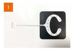
Place your cEEGrid in the applicator tool with the electrodes facing upwards.
