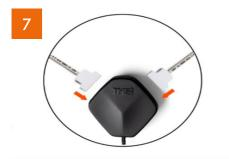
Once the grids are placed behind the ears, connect the cEEGrid to the connector box by sliding the grid connector into the adapter cable. Pay close attention to the orientation; make sure the labeling is pointing upwards, as in the photo above.
