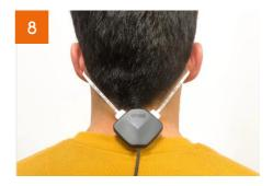
Connect the connecter box to a TMSi EEG amplifier, place your ground electrode, and begin measurements!
